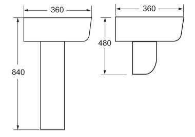
All measurements shown are in millimetres. Drawing sizes are not to scale. Measurement accuracy  $\pm$ 5mm. SONAS Bathrooms reserves the right to make changes and/or modifications to products and specifications without prior notice.
